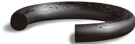
Figure 130 : Failure Due to Dieseling
