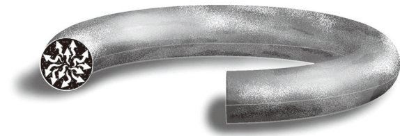
Figure 82: "Blooming" of the Internal Lubricant
