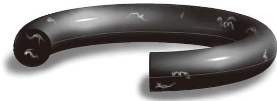
Figure 64: Embedded in the Seal
