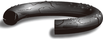
Figure 55: Failure due to Explosive Decompression
