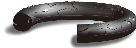
Figure 131: Failure Due to Explosive Decompression
