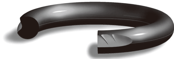
Figure 135: Failure Due to Installation Damage
