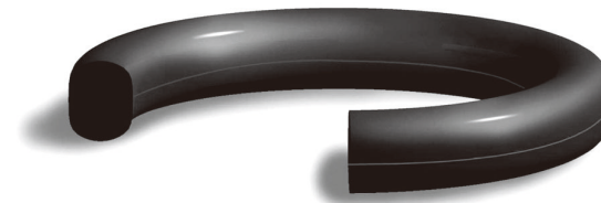
Figure 129 : Failure Due to Compression Set
