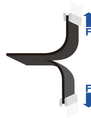
Figure 20: Slit ("Trouser") Specimen
