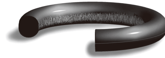
Figure 128 : Failure Due to Abrasion
