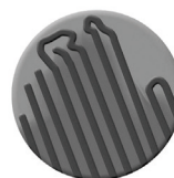
Figure 10: Linear, Symmetrical Chains
