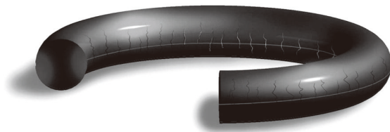
Figure 138: Failure Due to Weather & Ozone Cracking
