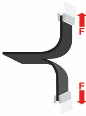
Figure 20: Slit ("Trouser") Specimen
