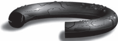
Figure 55: Failure due explosive decompression
