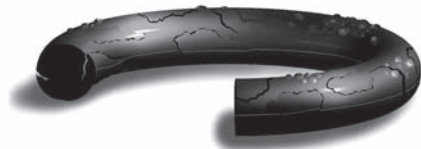
Figure 131: Failure Due to Explosive Decompression
